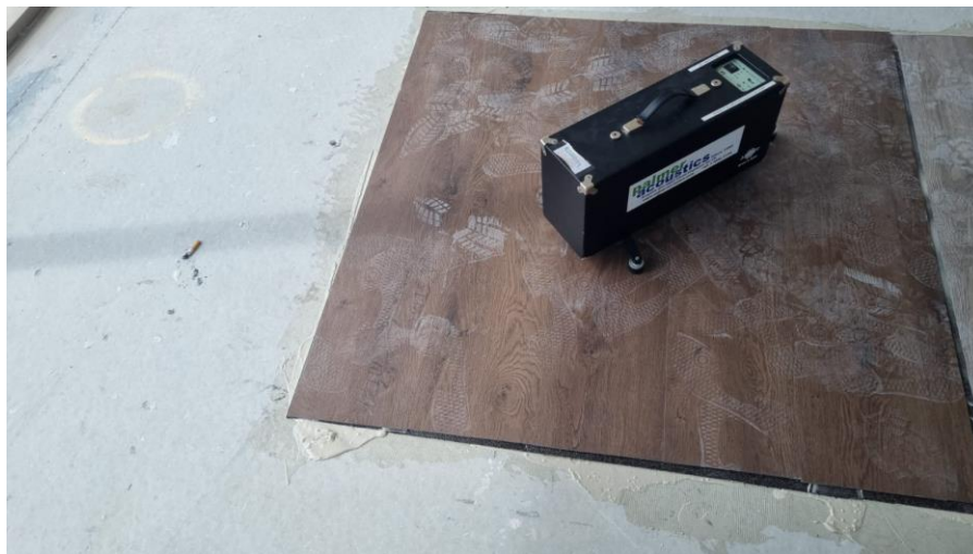
Figure 10: Test #10 – 4.5mm Vinyl Plank with 3mm GE Rubber Cork Underlay (Size 1200mmx1200mm)
