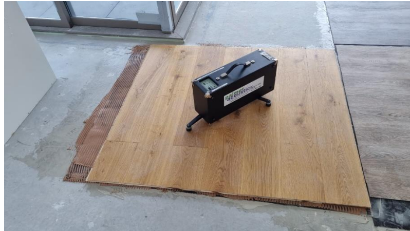
Figure 7: Test #7 – 14mm Engineered Timber with 3mm GE Rubber Cork Underlay(Size 1300mmx1200mm)
