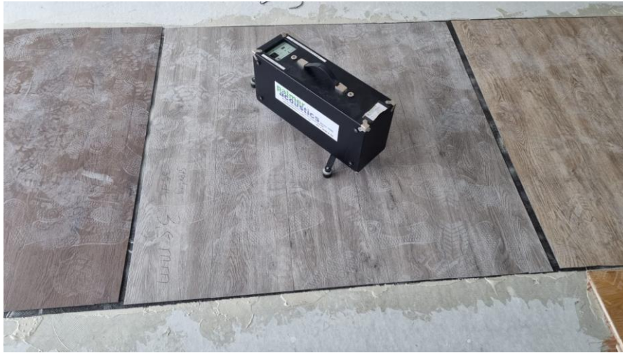
Figure 9: Test #9 – 3mm Vinyl Plank with 3mm GE Rubber Cork Underlay (Size 1200mmx1200mm)
