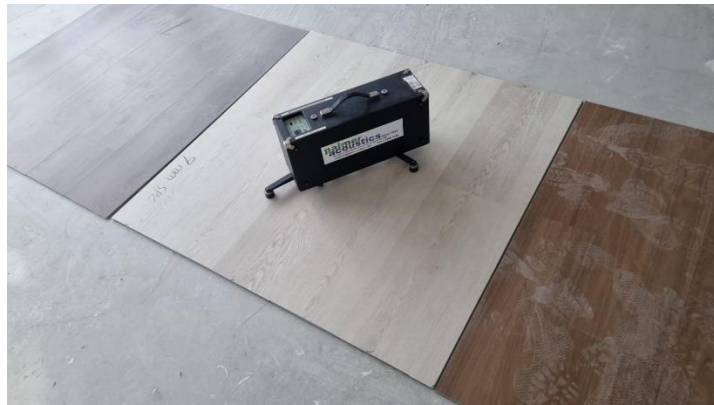
Figure 3: Test #3 - 8mm Hybrid SPC (Size 1200mmx1200mm)
