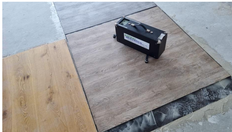
Figure 8: Test #8 - 5mm Vinyl Plank with 3mm GE Rubber Cork Underlay (Size 1200mmx1200mm)
