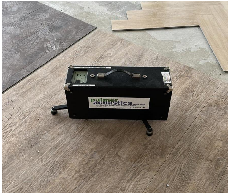
Figure 14: Test #14 - 5mm Vinyl Sample Floor (Size 1200mmx1200mm)
