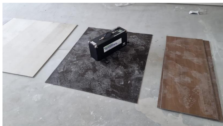
Figure 5: Test #5 3mm GE Rubber Cork Underlay (Size 1000mmx1200mm)
